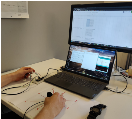
Figure 9 The participant holds the IMU in one hand for encoding. A sheet of paper containing the numbers helps with estimating the correct directions for encoding. The EMG (not visible) is placed on the left arm and can be used for resetting the last encoded number in order to increase accuracy and ITR. A comparison between EMG and non-EMG conditions can be seen in figure 14.
